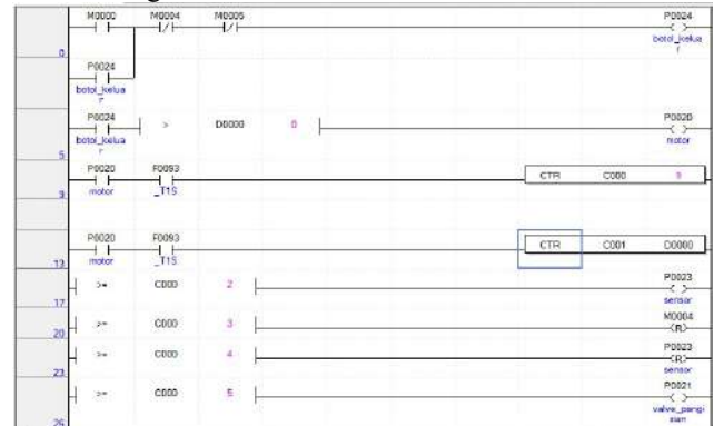
Gambar 5. Ladder Diagram Bottle Filling Process
